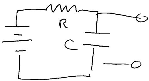
$$A(\omega) = \frac{V_{out}}{V_{in}} = \frac{1}{1 + i\omega RC}$$
