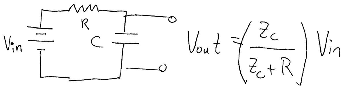
$Z_c = \text{impedance of the capacitor} = \frac{1}{i\omega C}$
